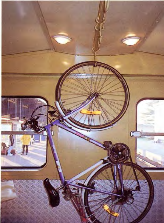
Hook system in a regional express train
